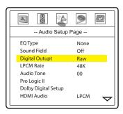
Due to bandwidth limitation of the technology and copyright restrictions, unfortunately it is impossible to send high-resolution multi-channel digital audio from a source like SACD or DVD-Audio to the receiver using this connection method. To enjoy SACD or DVD-Audio in their full resolution, please use the HDMI connection if you have a receiver that handles HDMI audio and use multi-channel outputs if you do not.
