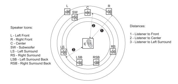
For example, in the above diagram, measure the distance (in feet) from the primary listening position to the Front Left or Front Right Speaker. Your Front Right and Left speakers should measure the same distance. If they do not, please adjust them if possible. Enter the distance of the Front Speakers (**1** in the above picture) using the left/right **ARROW** buttons.
