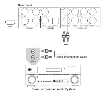
Method 8 – Stereo Analog Audio Connection
