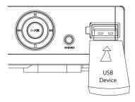
Please connect the USB device to the USB port of this DVD player using a compatible USB cable. Press the **DVD/USB** button on the remote control. A device selection menu will appear.
