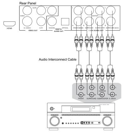
Receiver/Amplifier with 7.1ch Audio Input
